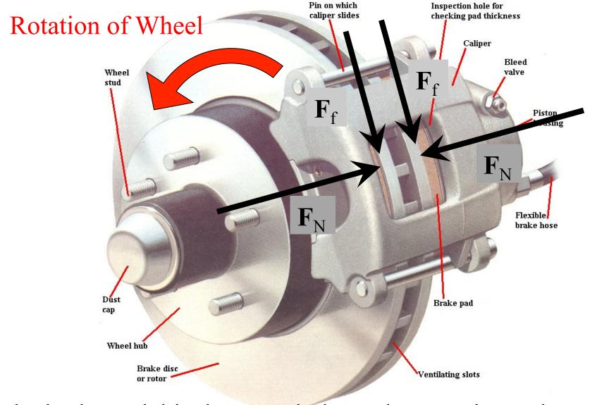
As the brake pedal is depressed, the pads move inward, creating greater normal force on the disc. This in turn produces greater friction opposing the rotation of the wheel.
