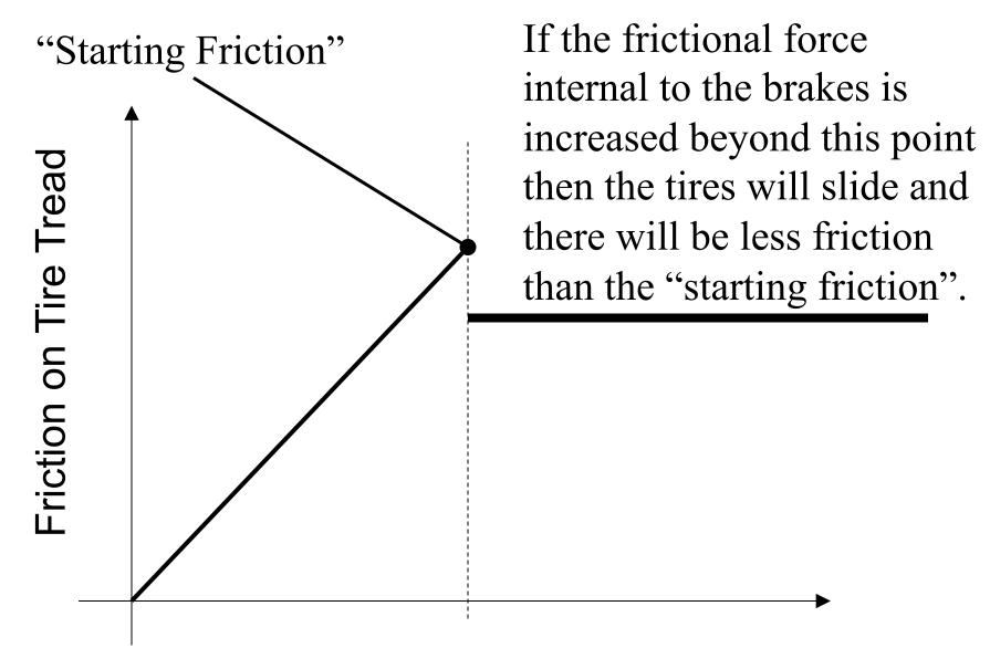
Friction on Disc Brake
